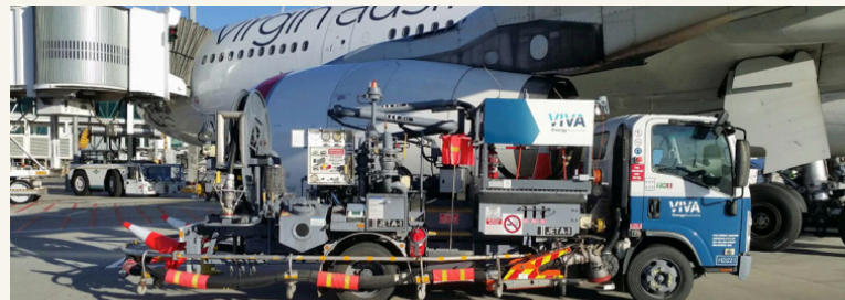
Newly branded Viva Energy Aviation hydrant cart
