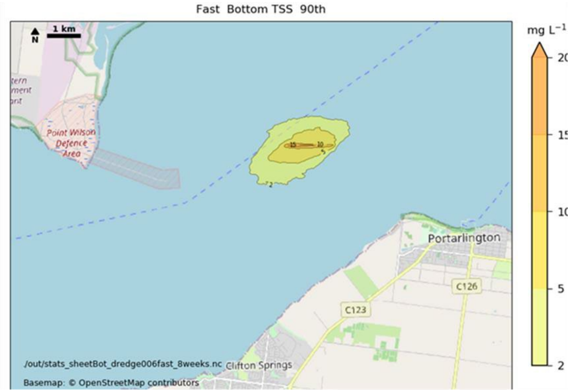
Figure 8-54 90 th -percentile total suspended solids concentration at the seabed – fast barge
