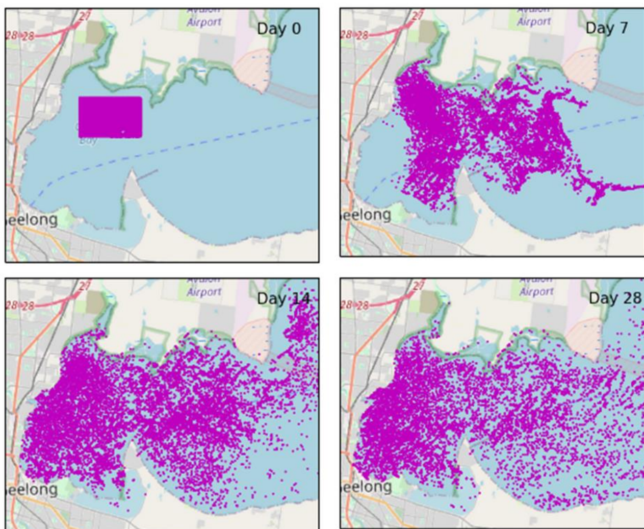
Figure 8-74 Distribution of particles from the north Corio Bay after 0, 7, 14 and 28 days
