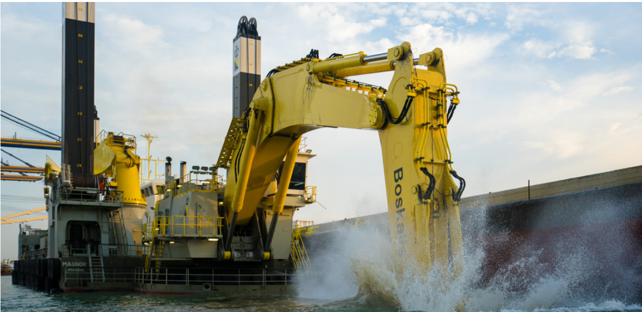
Figure 8-49 Example of dredging by a backhoe dredge (Source: Boskalis, 2021)
