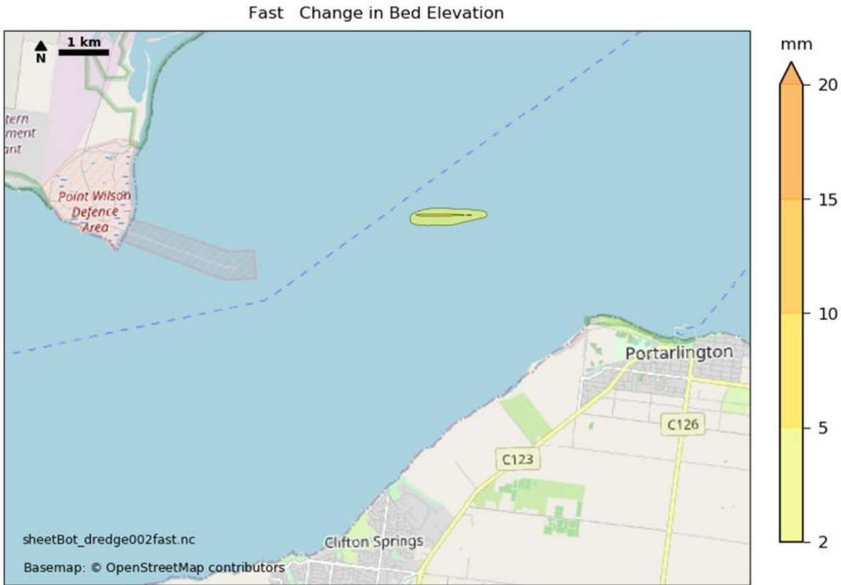
Figure 8-56 Changes in seabed elevation after 8 weeks with fast barge disposal
