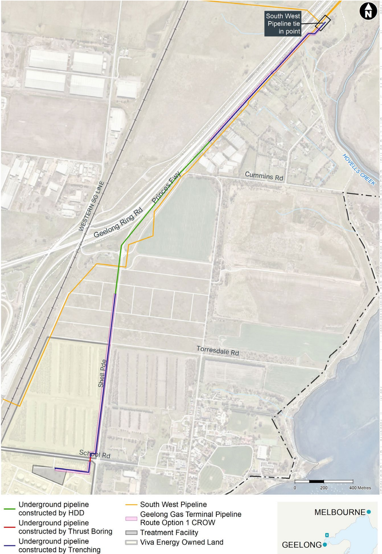
Figure 4-27 Proposed construction methodology for underground pipeline route sections
