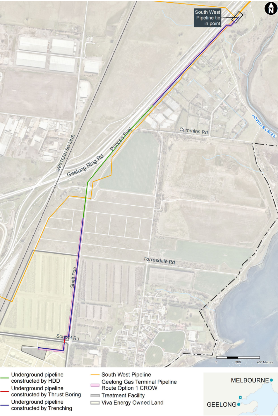
figure 2 Construction Trenching Map: Proposed location of trenching construction techniques for the underground pipeline including open trenching, HDD and thrust boring
