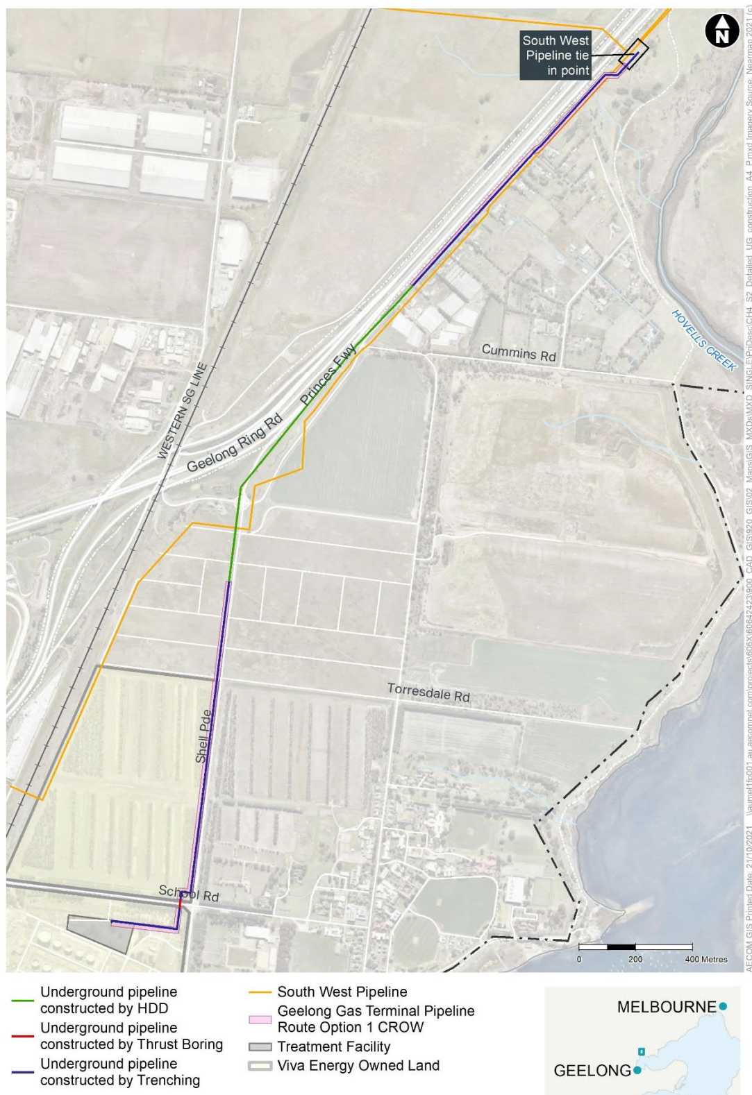
Figure 2: Proposed location of trenching construction techniques for the underground pipeline including open trenching, HDD and thrust boring
