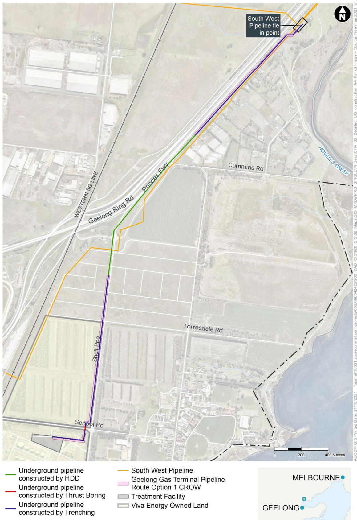
Figure 1-2: Proposed location of trenching construction techniques for the underground pipeline including open trenching, HDD and thrust boring
