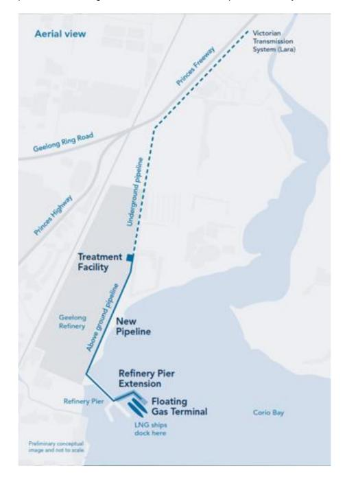
To the north of the Geelong Refinery along the proposed pipeline corridor, the area is predominantly rural. There are several other existing Viva Energy-owned underground pipelines running between the refinery and the connection point to the Victorian Transmission System at Lara.
