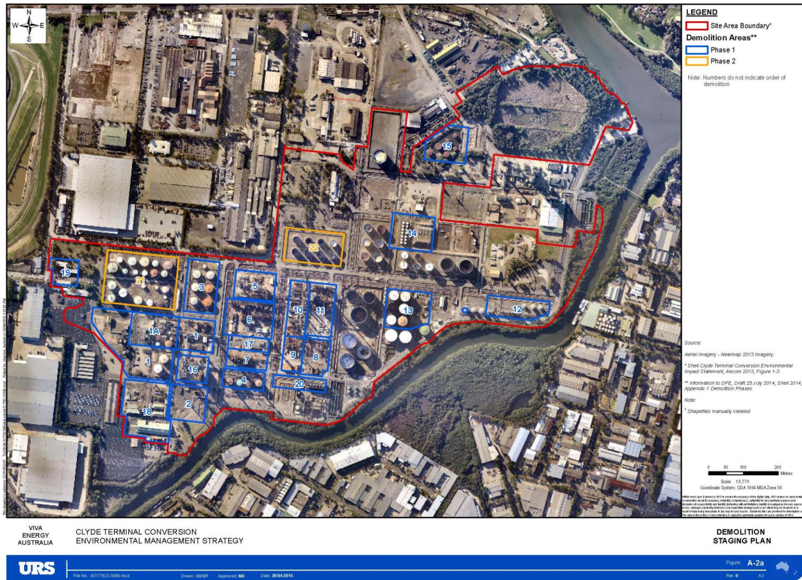
A.1 Figure A.1 Demolition staging plan
